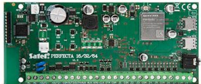
The PERFECTA 64 M control panel makes it possible to create wired and wireless systems – you can connect to it an **ABAX 2** system controller (**ACU-220** or **ACU-280** operating in the frequency band of 868 MHz) or **PERFECTA-RF**, i.e. the **MICRA** wireless system module (frequency band of 433 MHz). Alternatively, the **INT-RX-S** keyfob receiver expansion module may be connected to the control panel.
